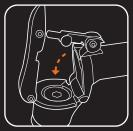
Lift the handlebar stem upwards, until it sits flat on the headset in the upright position.
