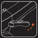
Connect the two halves of the frame together and secure by pushing the black locking handle into position firmly until you feel it click into its locked position.
