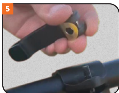
Replace the clamp handle making sure the brass washer is orientated correctly
