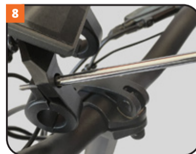
Remove screen mounting clamp screws
