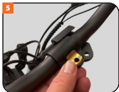
Reinsert the handlebar clamp
