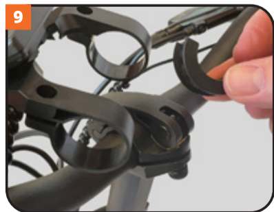
Remove mounting clamp spacers
