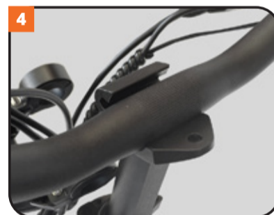
Place the handlebars exactly in the centre of the post
