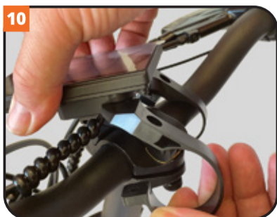
Gently open the mounting clamps and place over the handlebars
