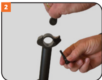
Remove clamp handle and tab
