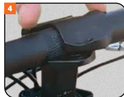
4 Place the handlebars exactly in the centre of the post
